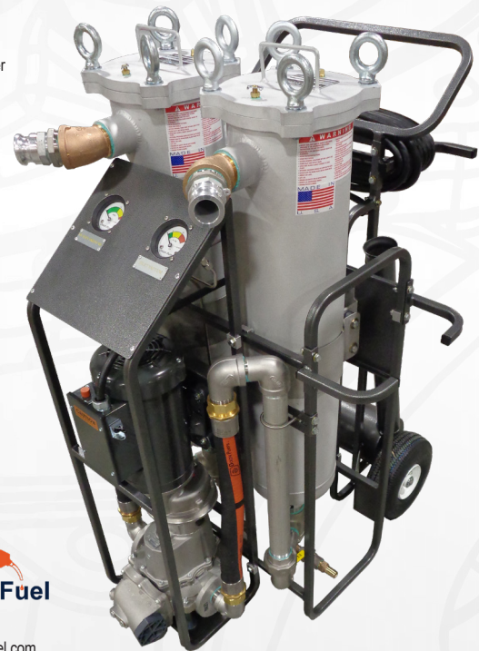
FS2 Mobile Filtration - 35 GPM - 2-Wheel Dolly - Inlet: Bag Filter, Outlet: Coalescing/Water Separation/Cartridge Filter
